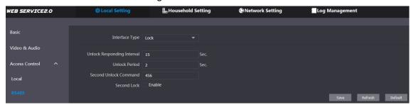
Step 2 Configure parameters, and you can select Lock or Lift Control in the Interface Type list. For the detailed description, see Table 4-4.
